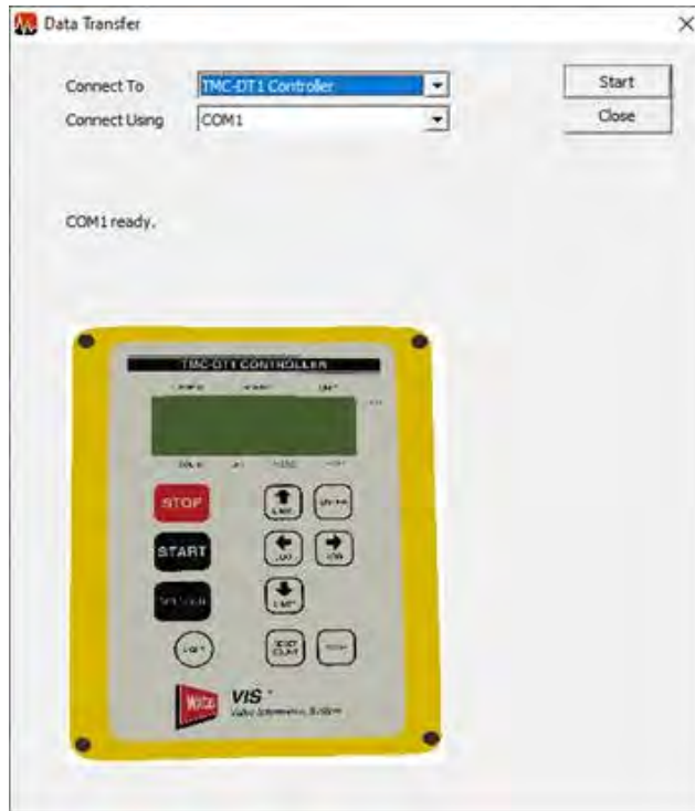
Figure 7-51. Data Transfer Start Screen for Yellow TMC-DT1 Controller.
