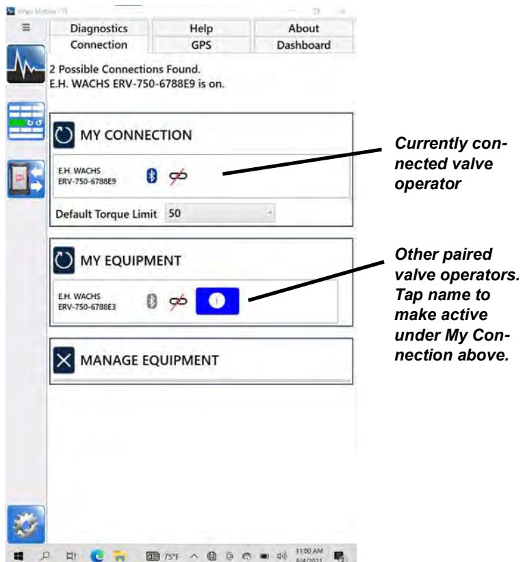
Figure 5-7. Connection Settings. A list of paired valve operators appears under MY EQUIPMENT . Tap the name to make it active under MY CONNECTION . (Only one is active at a time.)
