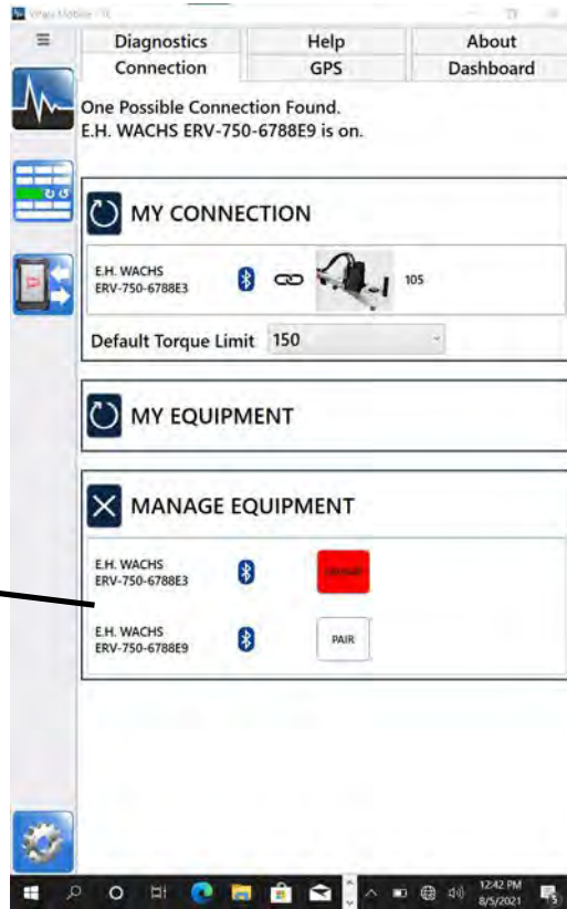
Figure 5-15. Display available valve operators under MANAGE EQUIPMENT .
