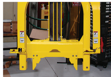
Guillotine saw shown with custom saddle for cutting steel I-beams, others available
