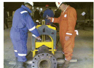
Guillotine saws feature fast, easy operation and the ability to cut most materials
