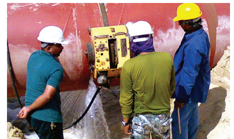
One Trav-L-Cutter can operate on multiple pipe diameters by adding additional chain sections
