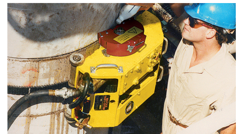
Highly versatile, the Trav-L-Cutter can cut vertically, horizontally or anything in between
