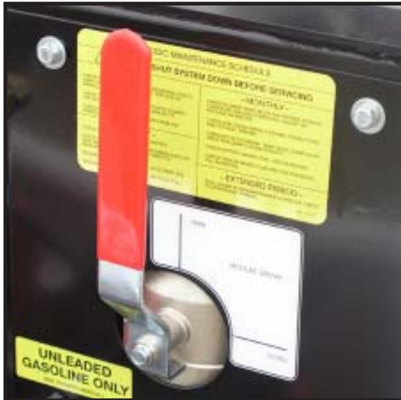
Vacuum break valve FIGURE 4
