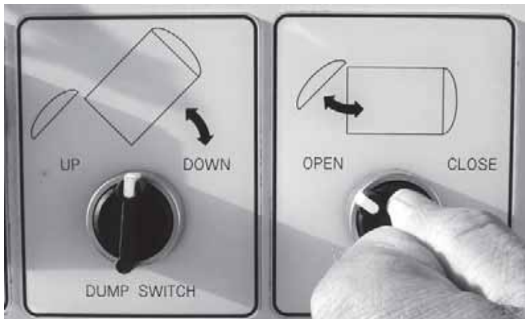
Figure 4-14. Turn the Latch Switch to the OPEN position and hold it until the latch fully opens.
