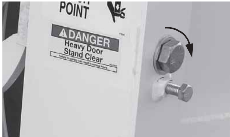
Figure 4-16. Turn the adjustment screw clockwise to tighten the latch.
