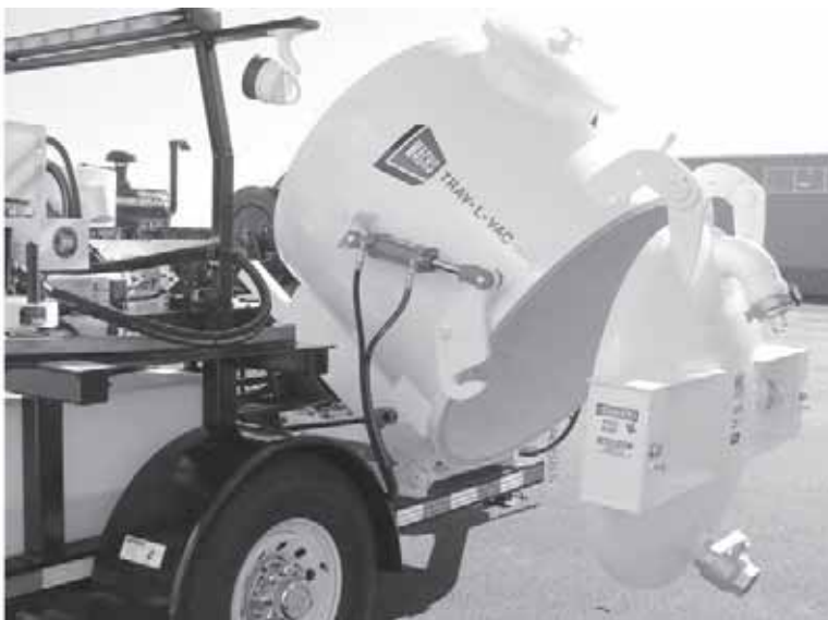
Figure 3-24. The tank door will swing open when the latches are released.
