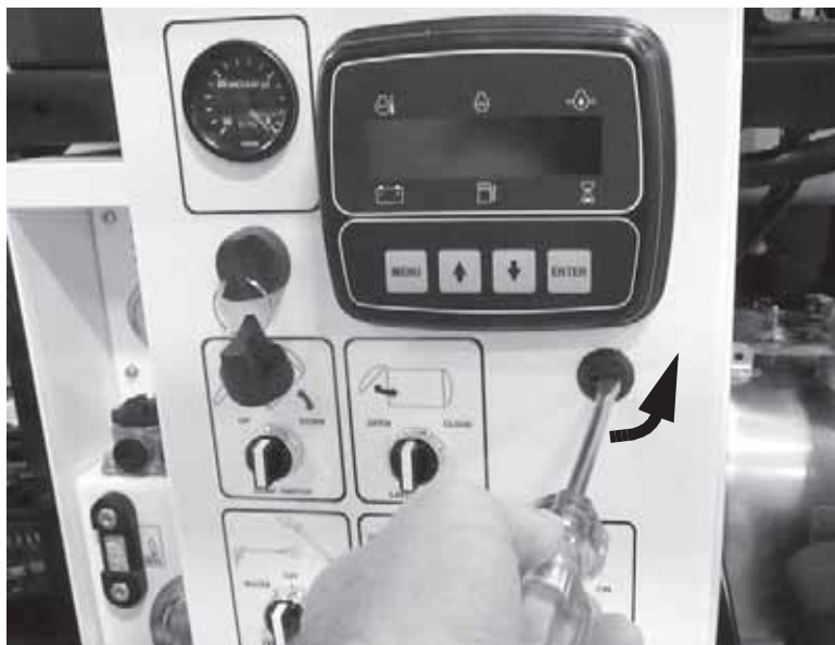
Figure 3-47. Use a screwdriver to open the control box and access the light bar control panel.
