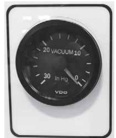
Monitor the pressure on the vacuum gauge while operating the vacuum.
