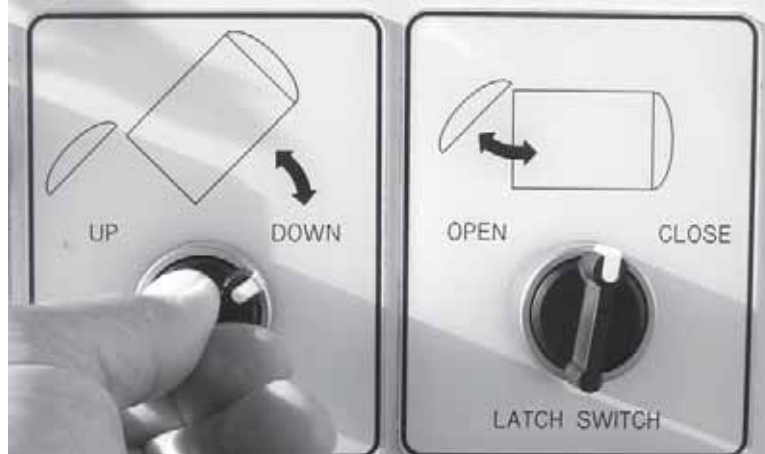
Figure 3-25. After the tank is dumped, turn the Dump Switch to the DOWN position until the tank has moved back to its operating position.
