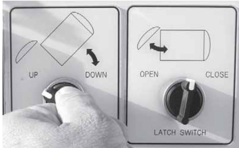
Figure 3-21. Turn the Dump Switch to the UP position and hold it until the tank is completely tipped.
