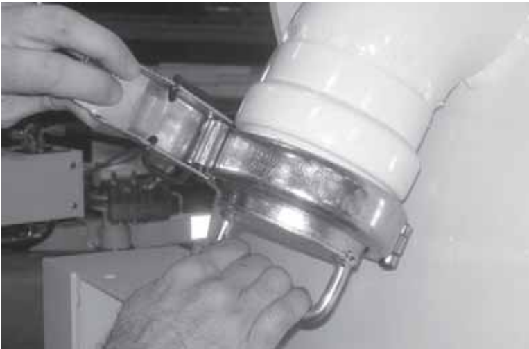
Figure 3-9. Pull the latch on the locking collar to release it and take it off the inlet port.
