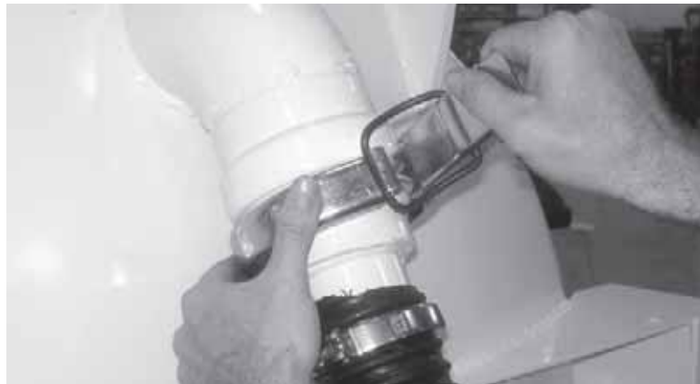
Figure 3-11. Insert the hose fitting into the inlet port and attach it with the locking collar.
