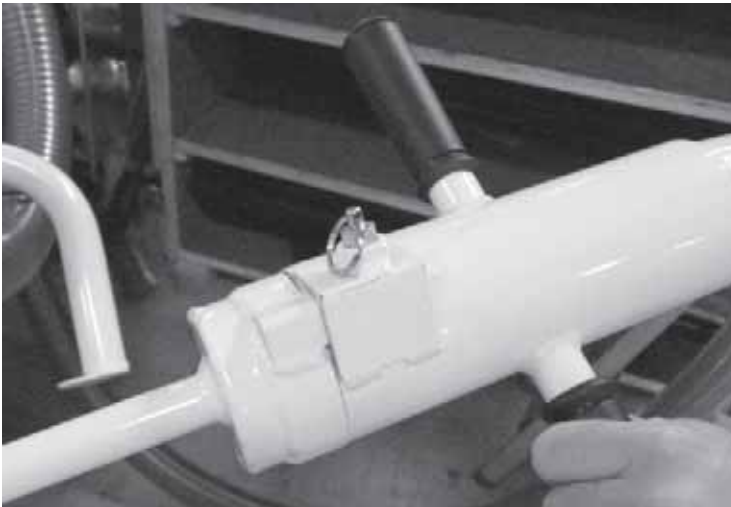
Figure 3-13. Insert the elbow into the wand until the lock pin engages to secure the wand.
