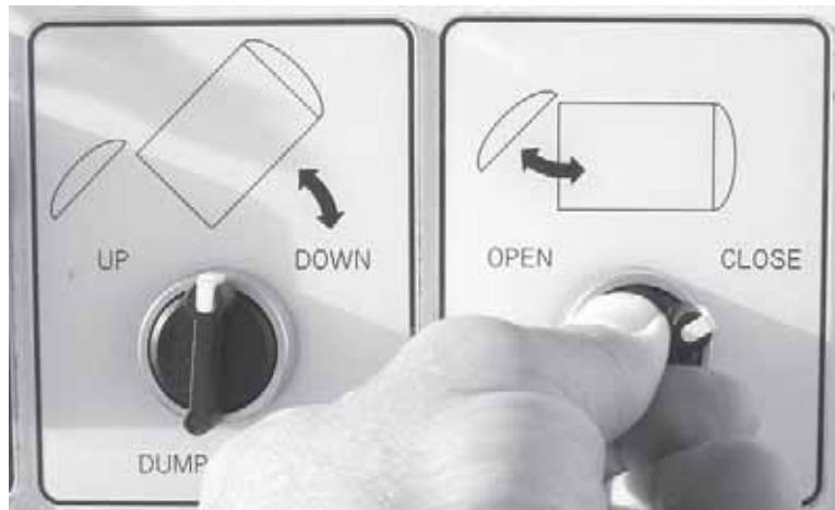
Figure 3-26. When the tank is in the down position, turn the Latch Switch to the CLOSE position until the latches are fully engaged.
