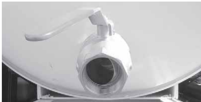
Figure 3-19. Check the drain valve before closing it to make sure there are no obstructions.
