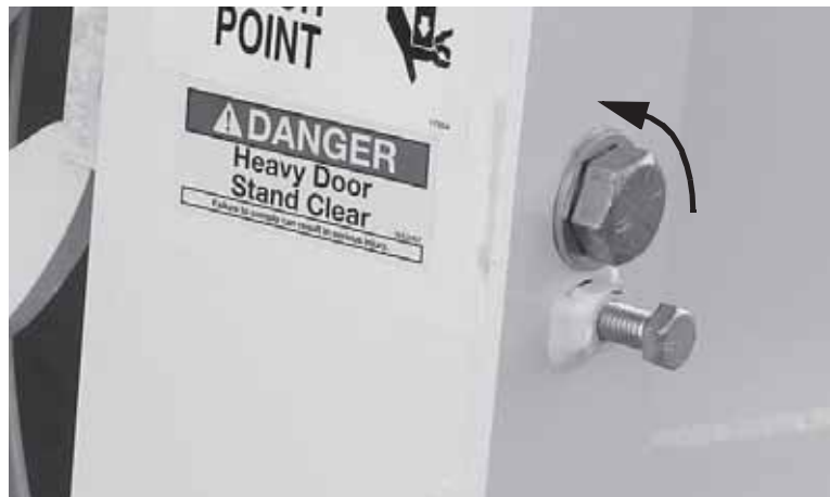
Figure 4-17. Turn the adjustment screw counter-clockwise to loosen the latch.
