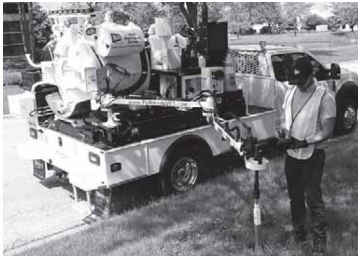
Figure 1-7. The ERV-750 valve operator extends on a telescoping swivel arm.
