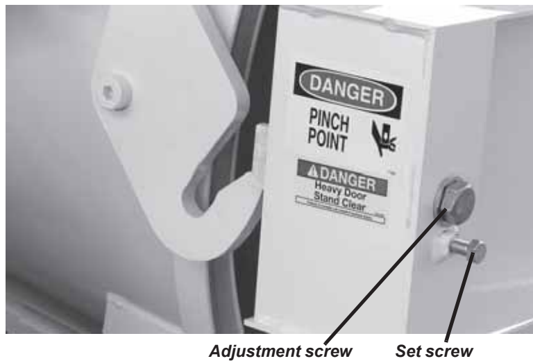
Figure 4-13. The front of the latch cover has screws for adjusting the latch.
