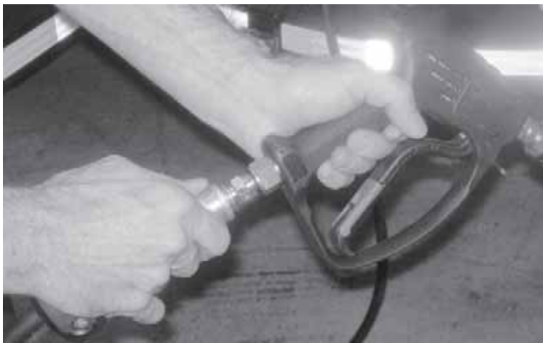
Figure 3-34. Attach the spray wand to the sprayer hose.
