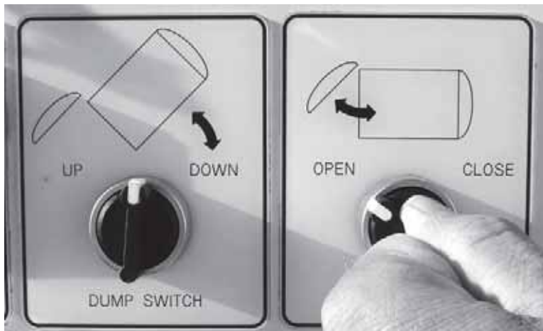
Figure 3-23. Turn the Latch Switch to the OPEN position and hold it until the door swings open.
