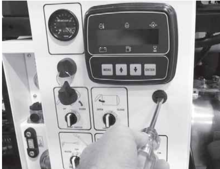
Figure 4-4. To access the fuse block, open the front of the curbside control panel.
