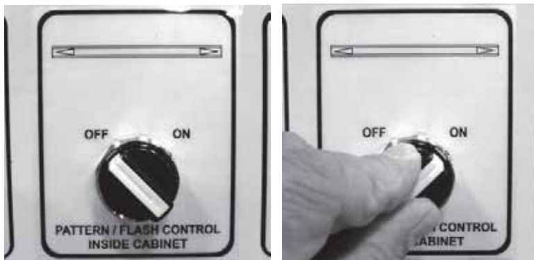
Figure 3-46. Turn the PATTERN/FLASH CONTROL switch ON to power the light bar.
