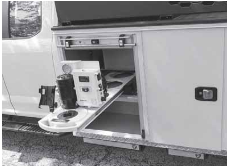
Figure 3-52. Loosen the lock knob on the side of the TM-7 slide rail, and pull the TM-7 out to the operating position as shown. Tighten the lock knob.
