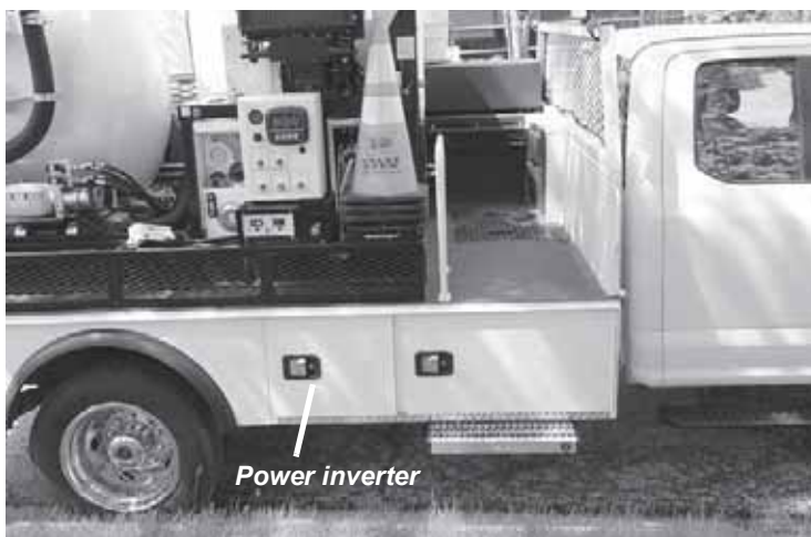
Figure 3-49. Open the cabinet door to access the power inverter.
