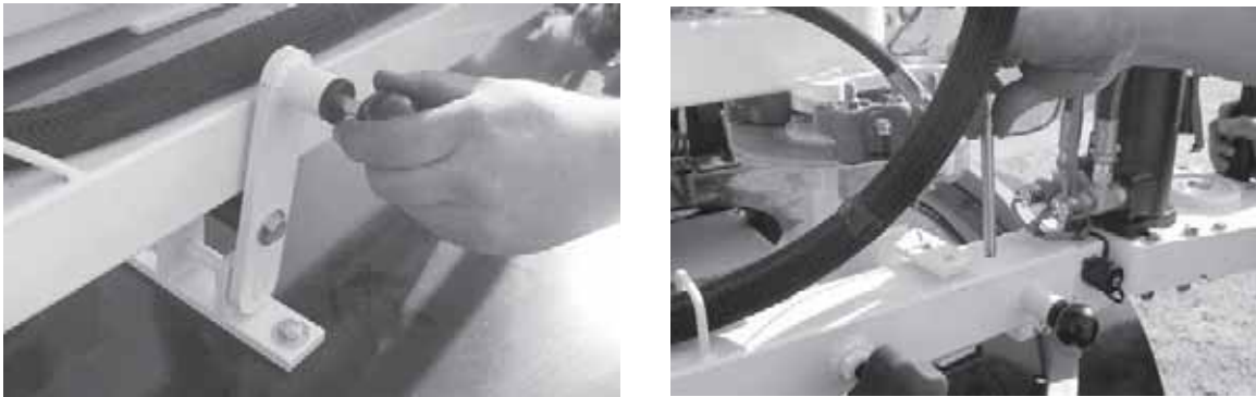
Figure 3-8. Release the two latches that secure the ERV-750 arm to the truck.
