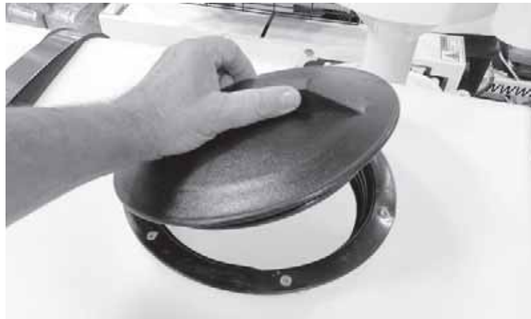
Figure 3-30. You can remove the lid from the top of the water tank to fill it.
