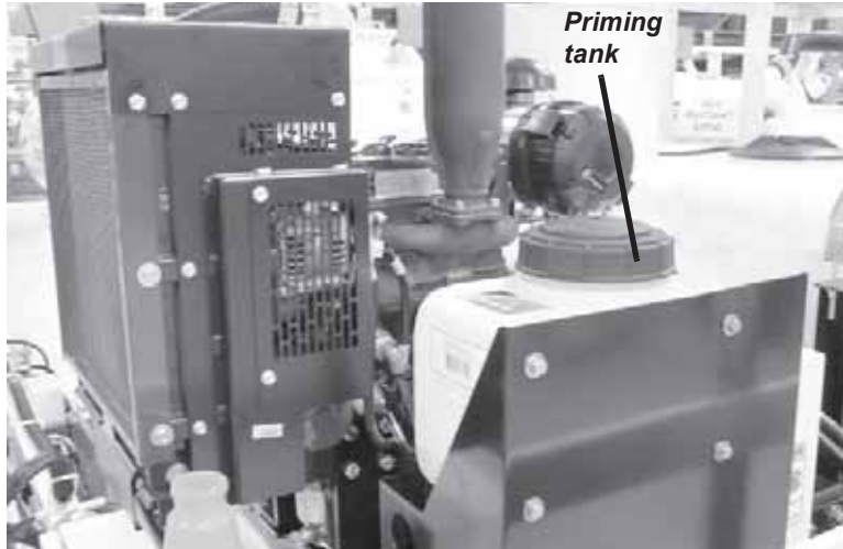
Figure 3-39. Remove the lid to fill the priming tank.
