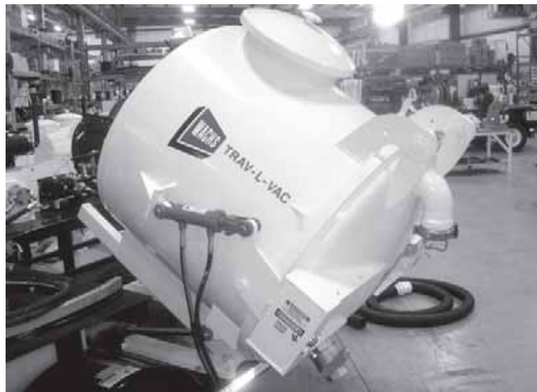
Figure 3-22. Tip the tank fully before opening the tank door.
