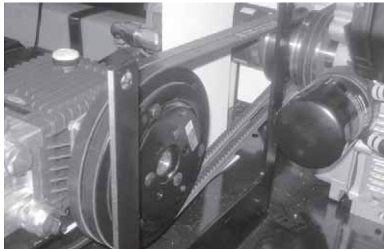
Figure 4-10. Inspect the sprayer pump belts for damage and correct tension.
