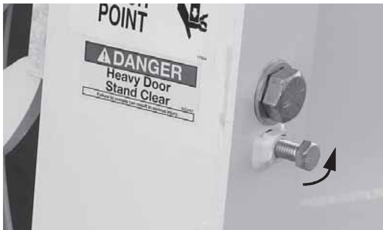
Figure 4-15. Turn the set screw counter-clockwise to loosen it.
