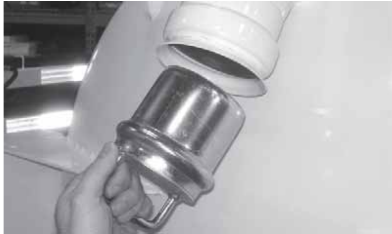
Figure 3-10. Remove the plug from the inlet port.
