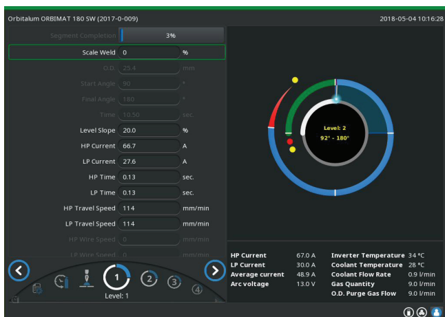
Fig. 13: Display during running welding process
