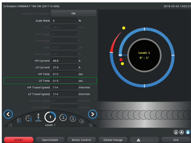
Fig. 18: Input field of a sector with representation of the seam scale
