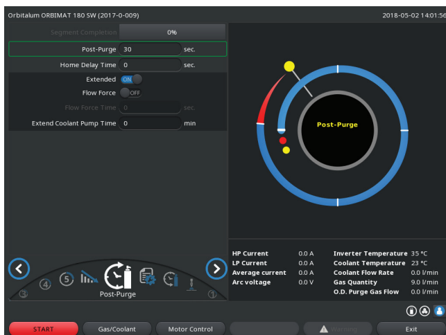
Fig. 15: Input field – Gas post purge time
