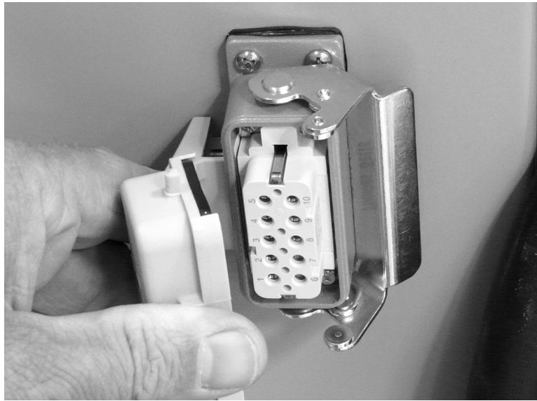
Figure 3-4. Attach power to the connector on the electrical panel of the HPU-20.
