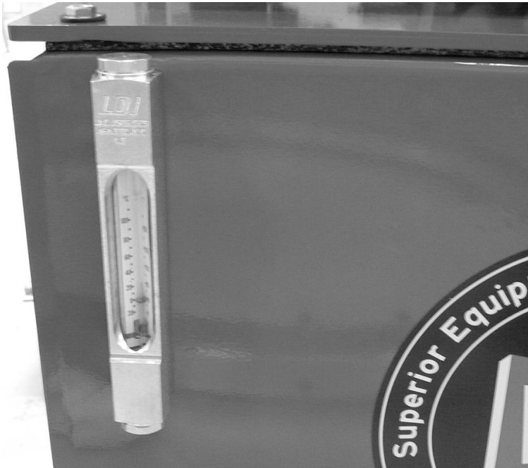
Figure 3-3. Fill the reservoir to the level indicated on the oil level/temperature gauge.
