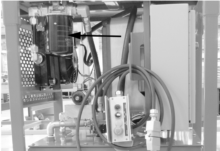
Figure 3-10. Replace the hydraulic oil filter every time you replace the hydraulic oil.
