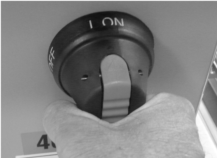
Figure 3-6. Turn the main switch on the front of the cabinet to the ON position.
