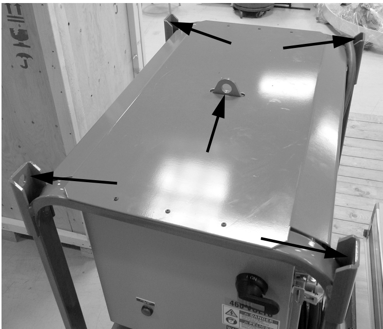
Figure 3-1. Use the lift points on top of the frame.
