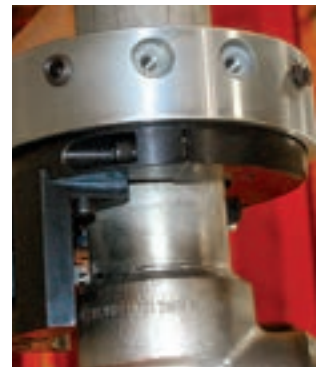
Axial Socket Weld Removal
