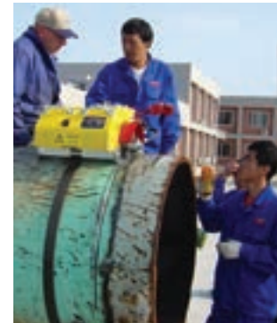
Trav-L-Cutter accommodates large diameters by adding chain sections
