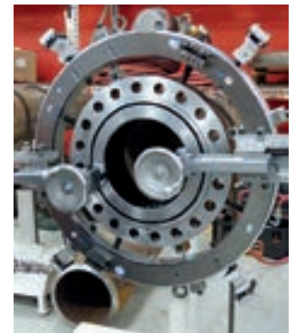
Two FFC modules simultaneously machine bolt face & record groove
