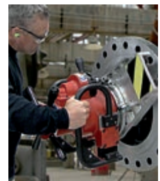
Faces flanges up to 36in (914mm) with optional slide
