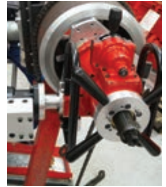
EP 424 SpeedPrep™ deluxe beveling with form tool rotating head
