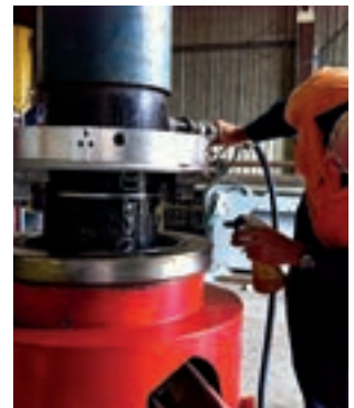
ECC can be used inverted for cut lines close to the flange
