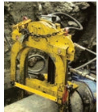
Elliptical cutting action, long blade life
