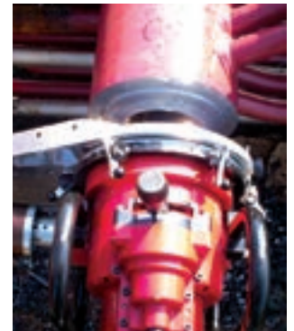
EP 424 SpeedPrep™ deluxe prepping heavy wall pipe
