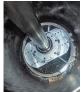
Internal cutting module lowered to cutting depth
