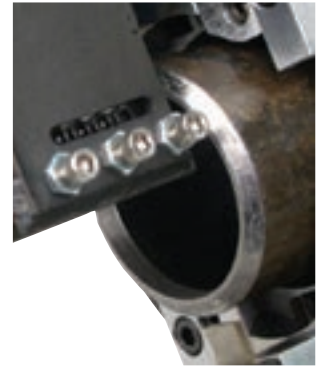
Counterbore attachment fits all models
