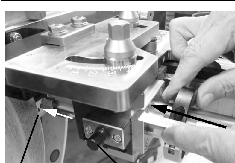
Set tool bit along OD to desired cut pass depth
