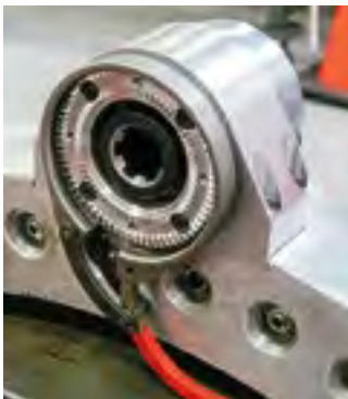
Tool-free drive mounting on heavy duty pinion to handle more power
