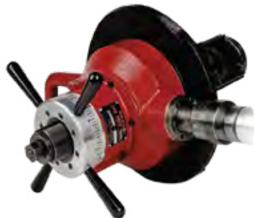
SDB End Prep performs pipe end preps & can be converted for flange facing
