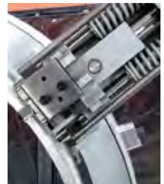
OD tracking slides follow out-of-round pipe & vessels.
