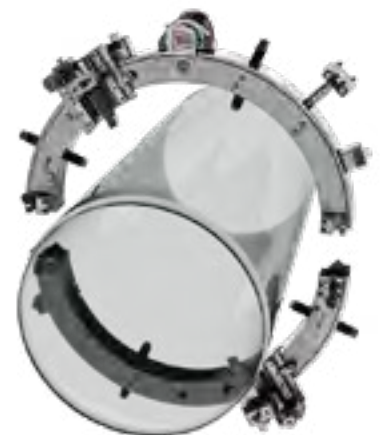
V-Lock ring mating surface resists force distortion
