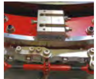
Swing bolts & hinge mechanism speeds assembly & mounting
