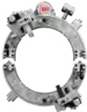
MDSF Split Frame unbolted for inline mounting
