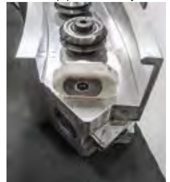
V-Lock ring mating surface resists force distortion
