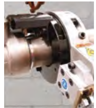
Socket Weld Removal
