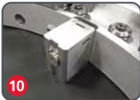
Clamp pads mount axially without removing the machine from the pipe
