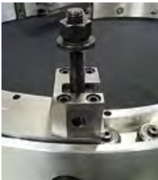
Aluminum stationary frame with steel rotating ring
