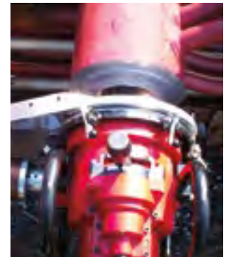
EP 424 AutoFeed deluxe prepping heavy wall pipe
