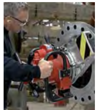
Ideal for facing flanges when properly equipped
