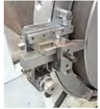
Slides feature Rapid Adjust and Micro Adjust
