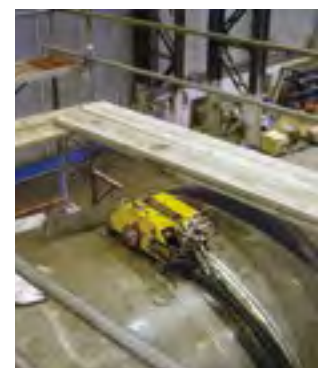
Trav-L-Cutter being used for submarine decommissioning
