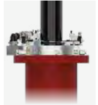
ECC simultaneously cuts and bevels casing
