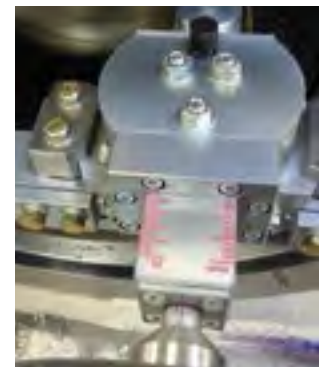
Modules are clearly marked to indicate depth and prep angle
