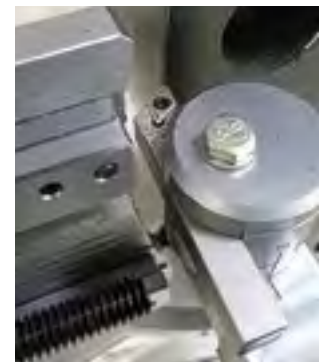
FFR tooling can be adjusted on multiple axes
