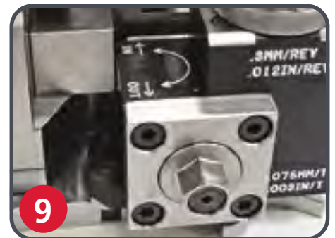
Rapid Adjust feature speeds positioning of tooling
