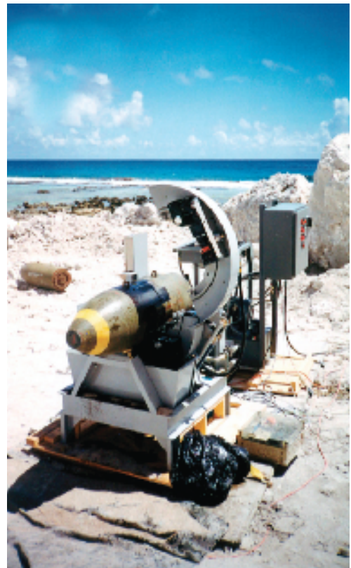
Fig. 6 – Automated cutting technologies used for demilitarizing WWII aerial bombs in Guam.
