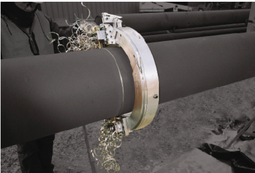
Fig. 4 – Versatile split frame machining systems utilize lathe technology to deliver perfect preps.
